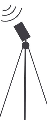
Noise from a sound source is measured across a proscribed frequency spectrum in both source and receiving rooms. The difference between the two measurements is the Sound Reduction Index (SRI)
