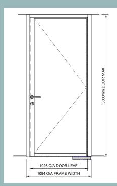
Elevation showing D660 door frame and ELITE Affinity 100mm door with lever handles
