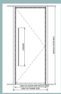
Elevation showing D660 door frame and ELITE Symmetry 100mm door with pull handles
