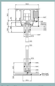
Top: Fixed 50mm head track at PSD opening Bottom: Floor guide track (carpet) at PSD opening
