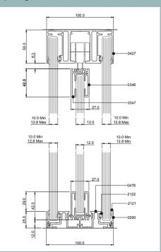
Top: Fixed 50mm head track at PSD side screen. Bottom: 25mm floor guide track at PSD side screen
