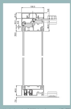
Vertical section D660 door frame and ELITE Vertical section D660 door frame and ELITE Symmetry 100mm door with pull handles
