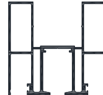
0445xxxxxxx PSD Lower Deflection Head (±40mm) 3100mm lengths Supplied as part of an ELITE Aero PSD kit Use with Internal Deflection Head (0442) and External Deflection Head (0443)
