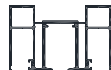
0428xxxxxxx PSD Lower Deflection Head (±25mm) 3100mm lengths Supplied as part of an ELITE Aero PSD kit Use with Internal Deflection Head ( 0412 ) and External Deflection Head ( 0426 )
